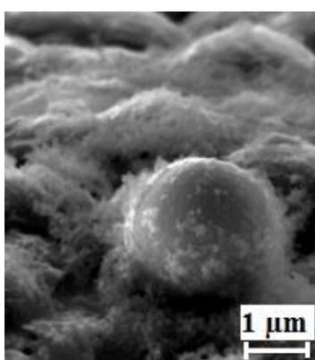
Figure 2: SEM image of diamond film on the globular stage
