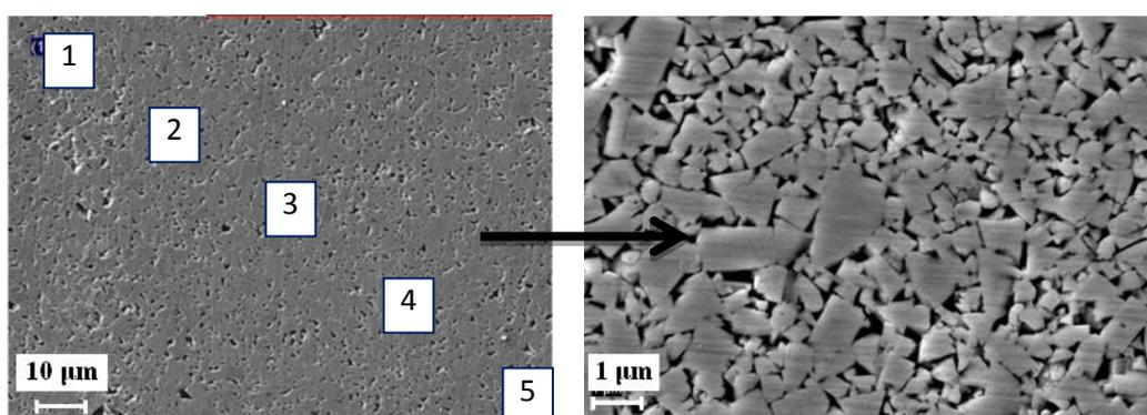
Figure 1: SEM image of the surface tungsten carbide of after a three-stage etching
