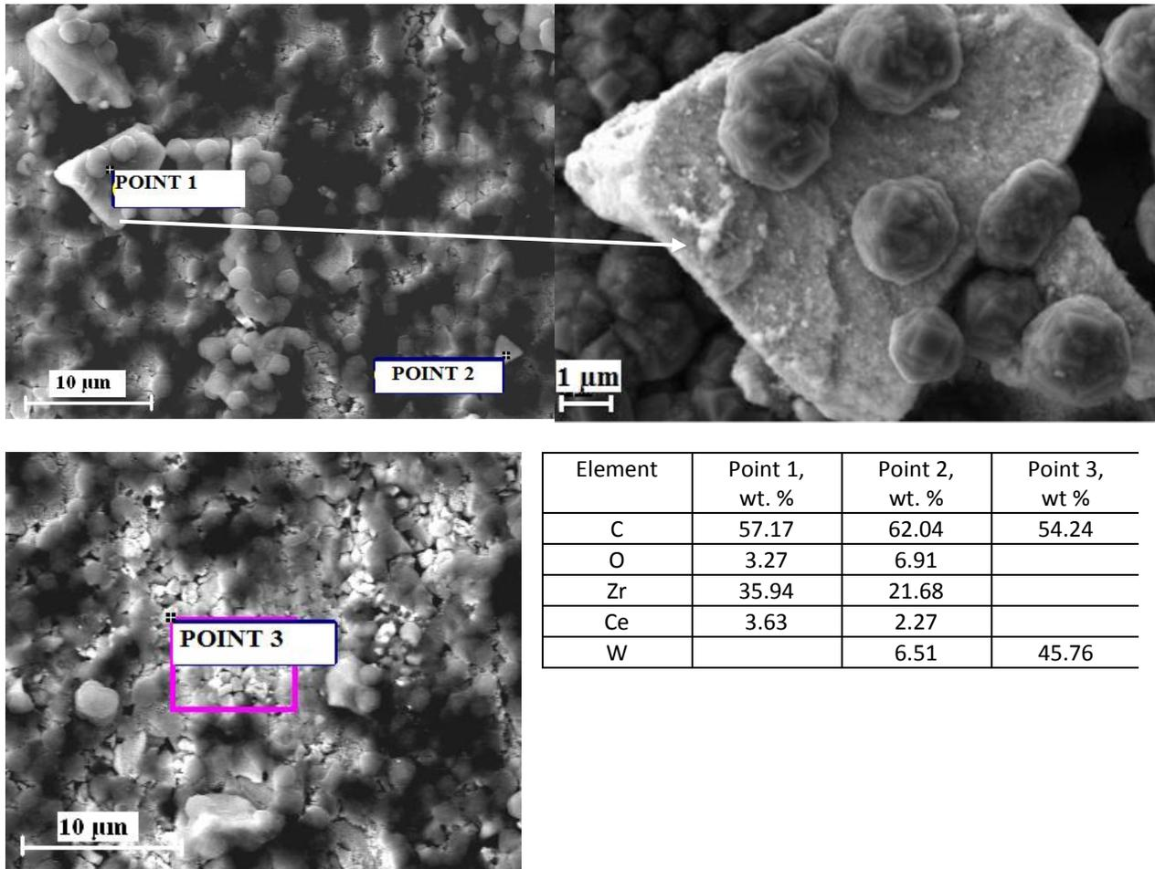
Figure 3: EDX –analysis of tungsten carbide surface of diamond film on the globular stage
