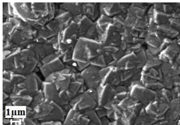
Figure 6: SEM images of diamond film on the stage of geometric selection
