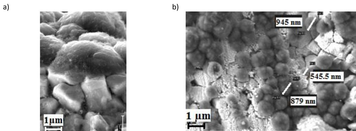
Figure 4: SEM images of diamond film on the stage of local formation of globules on the tungsten carbide grains (a) and in irregularities of substrate surface (b)
