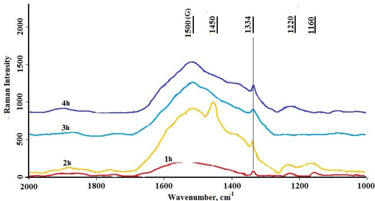
Figure 8: Raman spectroscopy of diamond film
