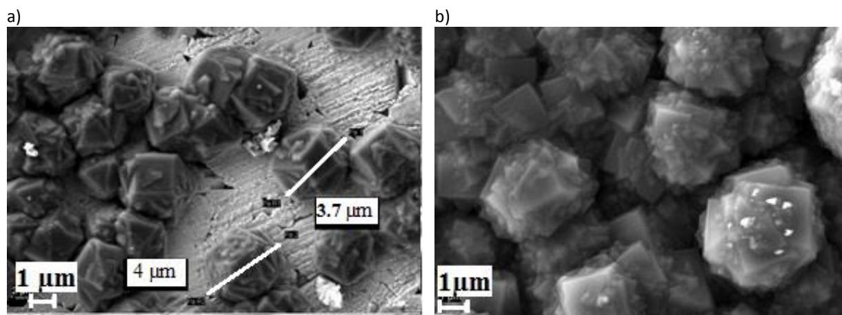
Figure 5 SEM images of diamond film on the stage of roughening of the globules structure (a) and their coating with numerous edges {100} (b)
